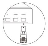
2. Gently push the module into the slot until you hear a click. Then, insert the RJ45 network cable.
